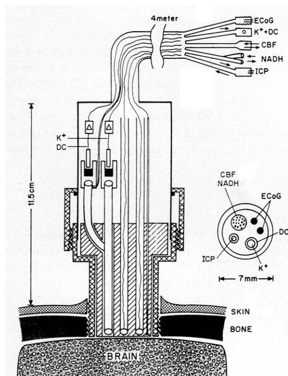
Fig. 1. The multiprobe assembly (MPA) used for monitoring the brain of head-injured patients. The MPA is connected to the brain via a special holder screwed into the skull. ICP, intracranial pressure probe; CBF, NADH, fiber optic light guide probe to measure local cerebral blood flow (CBF) and mitochondrial redox state (NADH);  $K^+$ , DC, extracellular  $K^+$  mini surface-electrode surrounded by a DC steady potential monitoring space; ECoG, bipolar electrocortical electrodes.
